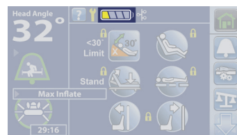
Touchscreen—Bed Battery Charge Level Indicator
