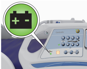
Caregiver Control Panel—Bed Battery Charge Indicator
